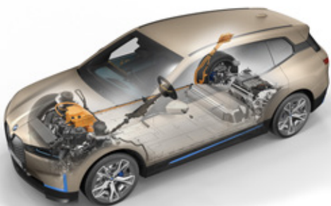
BMW 5 th generation eDrive with two motors
