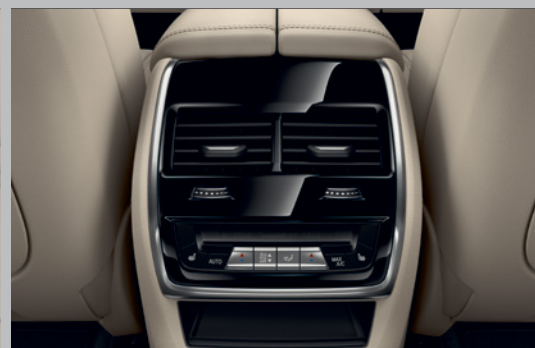
Automatic air conditioning with 4-zone control
